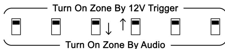
When the Turn On Options switch is set to "Audio/12V By Zone" you can set the six small 12V/Audio switches to select Audio or 12V turn on/off for each zone. For a zone that you wish to turn on and off by 12 volts, set that zone's switch to the up position labeled "Turn On Zone By 12V Trigger." For a zone you wish to turn on and off by audio, set that zone's switch to the down position labeled "Turn On Zone By Audio."
