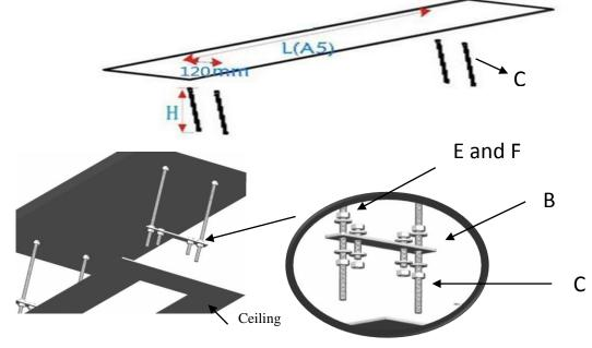
5. Push the screen up into the space. Use the **threaded rods** (C) to attach the screen assembly to the ceiling. The **hexagonal screws** (E) will connect the screen to the rest of the assembly. Once firmly in place; use the **nuts** (F) to ensure a firm connection. Use the **socket wrench** (D) to make sure that the
