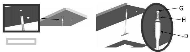
4. Insert thethreaded rods(C) through the M8 expanding bolts and then attach the M8x40mm hexagonal screwswith the washer (E). Last put the Hanging Bracket (B) through the threaded rod equal to the height of the screen's housing. Once they are firmly in place (as shown below) make sure that they will hold the weight of the screen.
