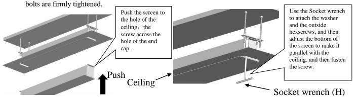
6. Install **end flange cover panel** (A) between the gap and the screen to complete the installation.
