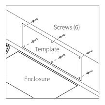
washers. We recommend that one person holds the subwoofer in place while another tightens the screws to secure the DSUB to the joist.
