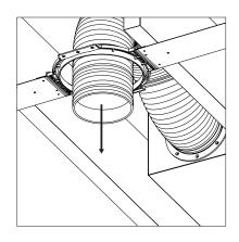
located close enough to the enclosure so that you will be able pull about 6" of the port tube through this hole.
